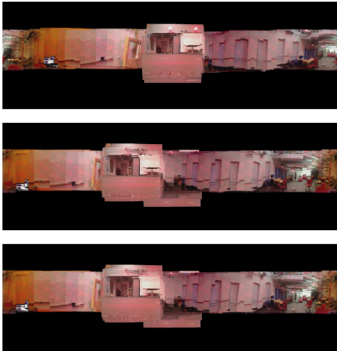
Fig. 9: (from top to bottom) Panorama stitches from VICON (ground truth) data, f -optimized, and f' -optimized orientations.
