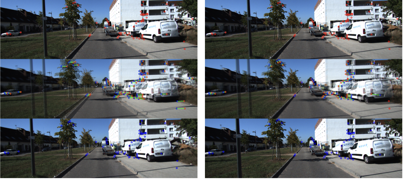
Fig. 1: Visual features matched across the left-right camera frames (left) and across time (right) (Source: ECE276A PR3 doc)
